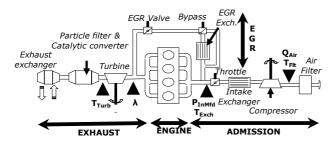
Fig. 3.Illustration of the diesel engine airpath system
