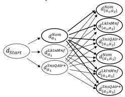
Fig. 6. Partial Markov Decision Process for the 3 faults and the final operation sequences  $\{a_1,a_2\}$  and  $\{a_1,a_3\}$ , with a highlight on the subpart starting from state  $d_{al}^{Nom}$ .
