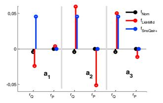
Fig. 4. Stem view of residual vectors for 3 faults  $f_{\text{Nom}}$ ,  $f_{\text{LklnMfd}}$  and  $f_{\text{SnsQair+}}$  and 3 static control actions  $a_1$ ,  $a_2$  and  $a_3$ . The y axis has no unit because residuals values are relative.
