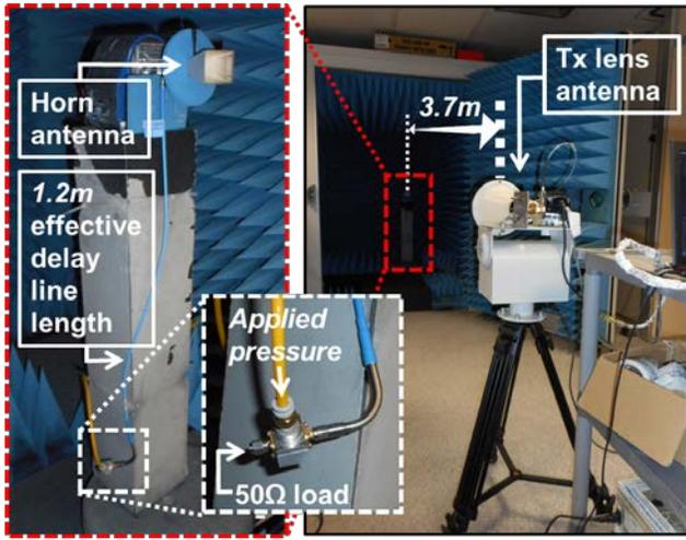
Fig. 5. Experimental set up for radar measurement.
