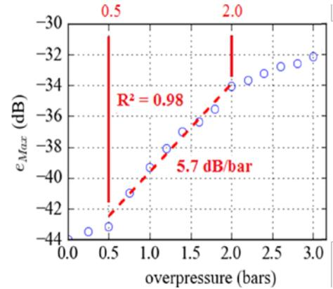
Fig. 8. Estimator  $e_{Max}$  (maximal echo level detected inside the scanned volume) as a function of the pressure applied on the passive pressure transducer. Between 0.5 and 2bars, a convenient linear variation is observed with a sensitivity of 5.7dB/bar and a coefficient of determination  $R^2$  of 0.98. The precision is estimated at 1.3% for  $e_{Max}=-42$ dB.
