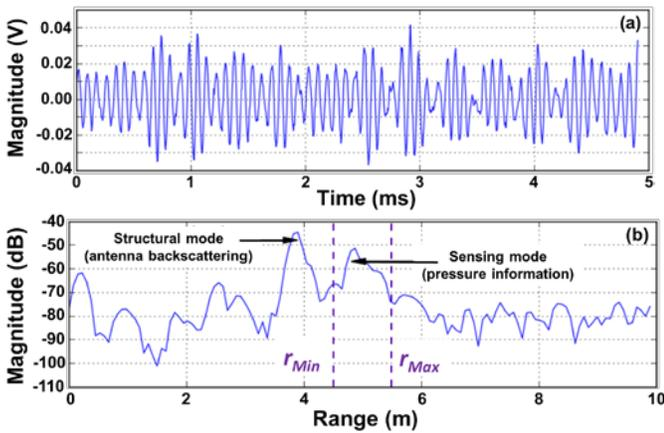
Fig. 6. (a) Time-difference signal and (b) beat frequency spectrum at a given direction of interrogation  $\theta=0^\circ$  and  $\varphi=0^\circ$ . Structural and sensing modes are characterized by two peaks separated by a distance corresponding to the effective length of the delay line. To retrieve the pressure, we focus on a range window between 4.5m and 5.5m noted  $r_{Min}$  and  $r_{Max}$ , respectively.
