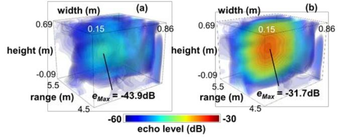
Fig. 7. 3D echo level of the passive pressure sensor displayed with isosurfaces (echo level with same values) for an overpressure of 0bar (a) and 3bars (b). The statistical estimator  $e_{Max}$  of the pressure is defined here as the maximal echo level detected inside the scanned volume.
