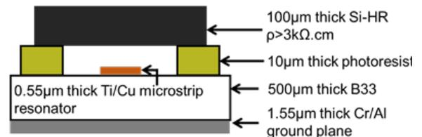
Fig. 2. Cross-sectional view of the different sensor layers.  $\rho$  denotes the resistivity parameter. Both relative permittivity ( $\epsilon_R$ ) and the loss tangent ( $\tan \delta$ ) of each material are given in Table I.
