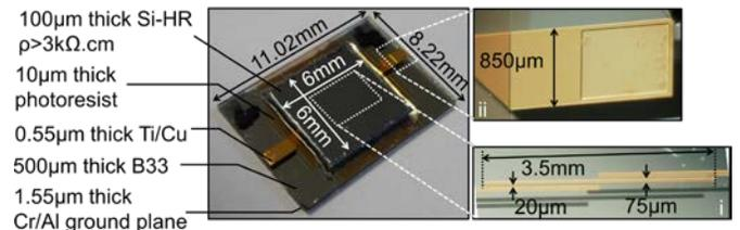
Fig. 1. Photo of the microwave sensor after bonding with its Si-HR membrane.  $\rho$  denotes the resistivity parameter. The insets (i) and (ii) show the microstrip half-wavelength resonator below the membrane and the input or output port (9 $\mu$ m thick Cu) of the resonator, respectively.
