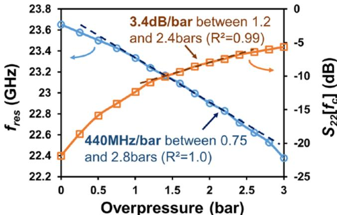
Fig. 4. Variation of the measured resonant frequency  $f_{res}$  and of the measured input reflection coefficient  $S_{ii}$  at  $f_c$  of 23.8GHz (radar operating frequency) as a function of the overpressure.
