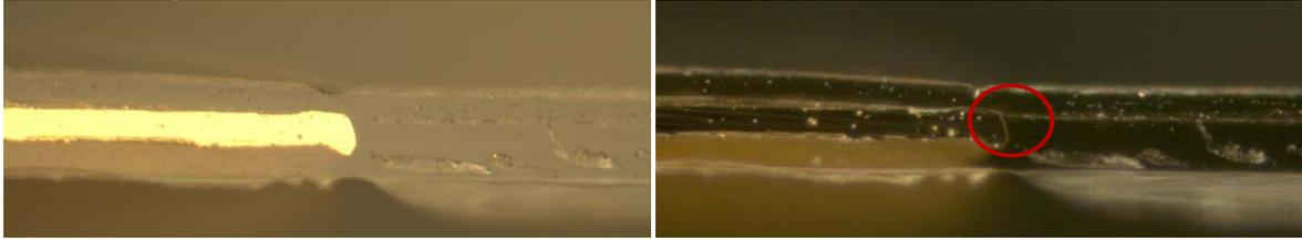
Fig.5 & 6: pictures of 9 $\mu$ m gold vias and the metallization line on the top
