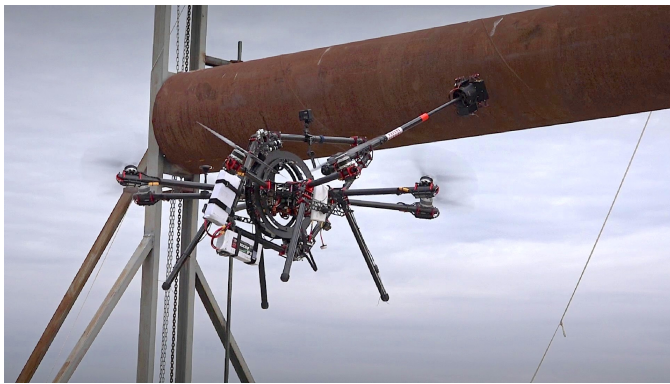
Fig. 10. Outdoor contact inspection experiments with AEROARMS aerial robot
