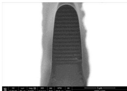
Figure 5 : dense nanowire network in a SU8 microfluidic channel, after removing the cover through a FIB etching.
