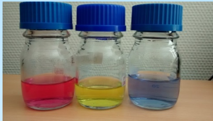
Quick 3-points calibration of ISFET in buffer pH solutions
