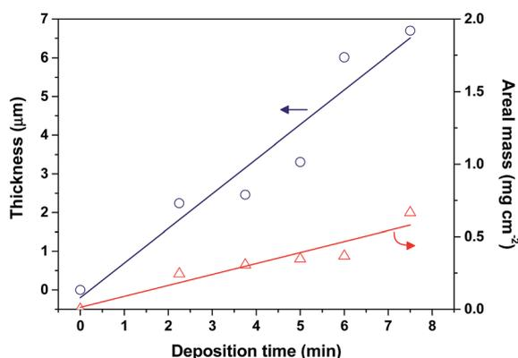
Fig. 2 Evolution of the thickness and the mass with deposition time for the  $\text{Li}_4\text{Ti}_5\text{O}_{12}$  deposits prepared at  $E = 32 \text{ V cm}^{-1}$  in a  $1 \text{ g L}^{-1}$   $\text{Li}_4\text{Ti}_5\text{O}_{12}$  suspension ( $0.1 \text{ g L}^{-1}$  of  $\text{MgCl}_2$ , 95% ethanol – 5% water).
