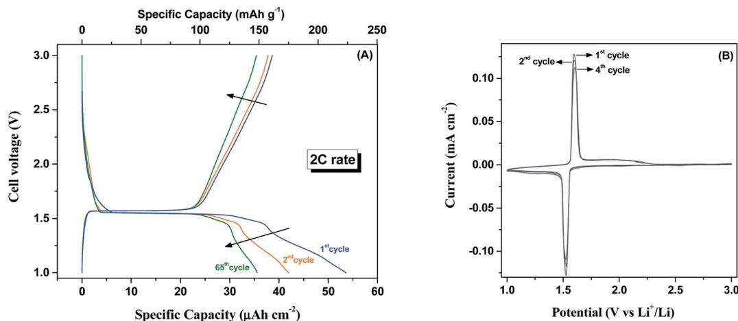
Fig. 4 (a) Galvanostatic lithium insertion/extraction profiles and (b) cyclic voltammogram recorded at  $0.1 \text{ mV s}^{-1}$  for the prepared  $\text{Li}_4\text{Ti}_5\text{O}_{12}$  electrodes.
