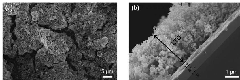
Fig. 1 SEM micrograph ((a) surface; (b) cross-section) of the  $\text{Li}_4\text{Ti}_5\text{O}_{12}$  deposits obtained at  $E = 32 \text{ V cm}^{-1}$  in a  $1 \text{ g L}^{-1}$   $\text{Li}_4\text{Ti}_5\text{O}_{12}$  suspension ( $0.1 \text{ g L}^{-1}$  of  $\text{MgCl}_2$ , 95% ethanol – 5% water) during 5 min.
