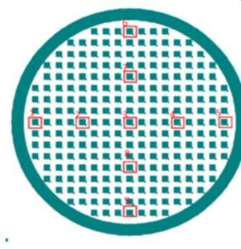
With this mask, we varied several parameters on each tool according to our bath restrictions before measuring thickness on 9 points ideally dispersed on the wafer, these measurements allowed us to determine the optimum parameters to reach the best metal distribution rate with ideally dispersed design:
