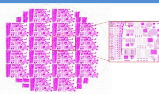
The second mask has design with different shapes (lines, squares, circles...) and sizes (from 5um to 60um) non-ideally dispersed on the wafer, according to micro fabrication processes with different sized components.
