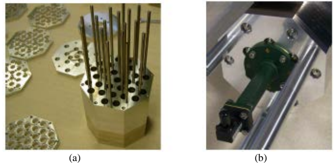
Fig. 20. (a) Mock-up assembly with the alignment of the milled layers (SAP Micro Mecanique©) and (b) transitions used to realize the linear excitation.
