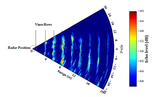
Fig 2. Two-dimensional polar plot of electromagnetic echoes from the vineyard (cut-plane  $\phi=0^{\circ}$ ). High echo levels allows locating the vines rows.
