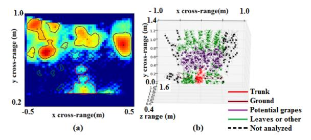
Fig 5. Echo level contours (a) in a cut-plane z=0.825m and (b) in the interrogated 3D space
