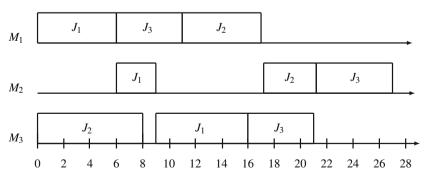
Fig. 9.2: Gantt representation of a solution to the job shop problem
