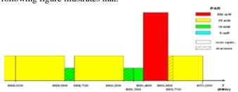
We use a statistical frequantial repartition to choose one frequency that will have the emitted signal. More precisely, inside each channel of 200 kHz which is centered on f<sub>c</sub>, the emitted signal will have a frequency that is far by f<sub>i</sub> from f<sub>c</sub>. The bandwidth of each emitted signal is around 100Hz which represents number of symbol bits emitted.
