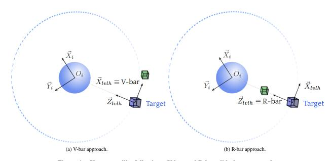
Figure 4 Chaser satellite following a V-bar and R-bar glideslope approach.
