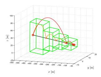
**Figure 10** Chaser relative trajectories: standard elliptic glideslope algorithm (red) vs. proposed optimal algorithm (orange).
