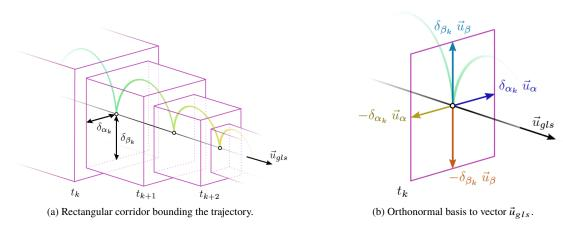
Figure 3 Glideslope corridor constraints.
