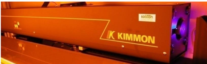
Figure 1: laser He-Cad, 442 nm, 125 mW
