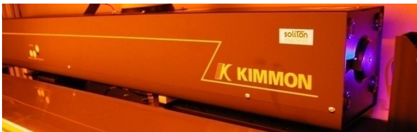
Figure 1: laser He-Cad, 442 nm, 125 mW
