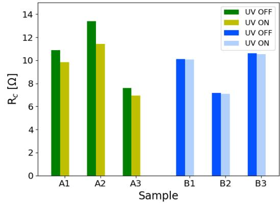
Fig. 9. Histogram showing the values of  $R_C$ , with and without illumination for the 6 samples of technologies A and B: with technological option A,  $\Delta R_C$  appears to be more much larger than that obtained with the technological option B.
