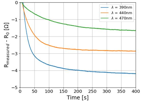
Fig. 3. Variations in the measured resistance as a function of time at several wavelengths.  $R_0$  represents value of the resistance in the dark.  $V_{TLM} = 200$  mV,  $T = 25$  °C, under an irradiance of few  $\mu\text{W}/\text{cm}^2$ .
