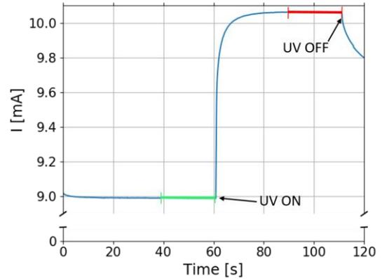
Fig. 6.  $I(t)$  curve used to calculate the two resistances in the dark (green bar) and under UV illumination (red bar) under an irradiance of few  $\text{mW}/\text{cm}^2$ , at  $T = 25 \text{ }^\circ\text{C}$ ,  $V_{\text{TLM}} = 500 \text{ mV}$ ,  $L_i = 16 \text{ }\mu\text{m}$ .
