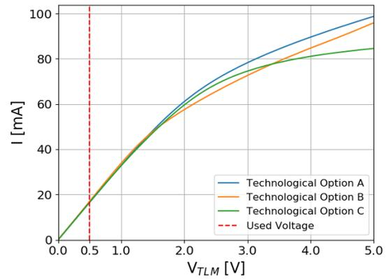
Fig. 5. I-V characteristics for three samples of each technological options, at  $T = 25 \text{ }^\circ\text{C}$ ,  $L_i = 4 \text{ }\mu\text{m}$ . The selected voltage is 500 mV for all following measurements (dashed red line).
