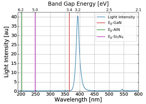
Fig. 2. Emission spectrum of the UV LED light used (blue), corresponding bandgap energy of: GaN (red), AlN (green), Si<sub>3</sub>N<sub>4</sub> (purple).
