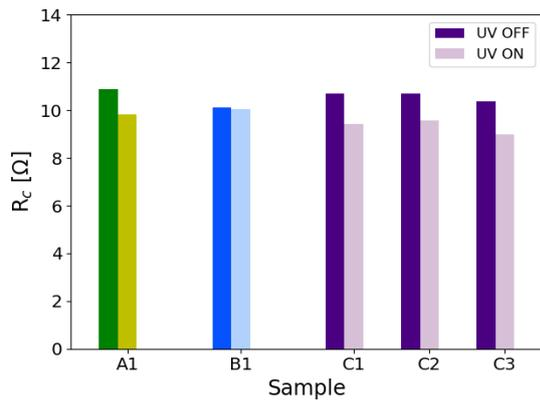
Fig. 10. Histogram showing the values of  $R_c$ , with and without illumination for some samples of technologies A, B and C: the samples of technological option C exhibit the same behaviour as those of technological option A in terms of  $\Delta R_C$ .
