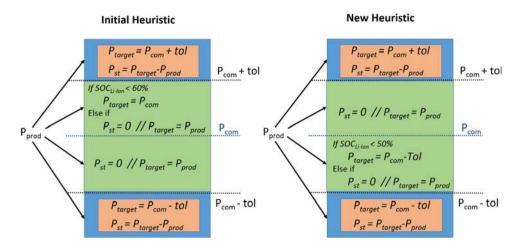
Fig. 8. New Heuristic algorithm.
