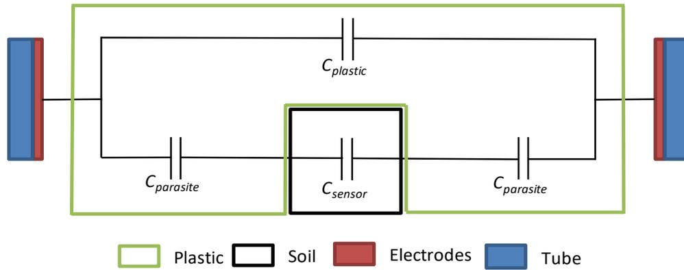
Figure 14. Model of the integration effect on the sensor
