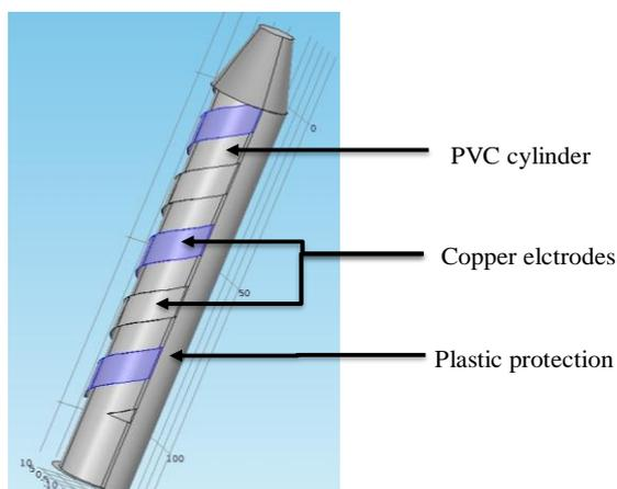
**Figure 5.** Sensor in the shape of a helicoid
