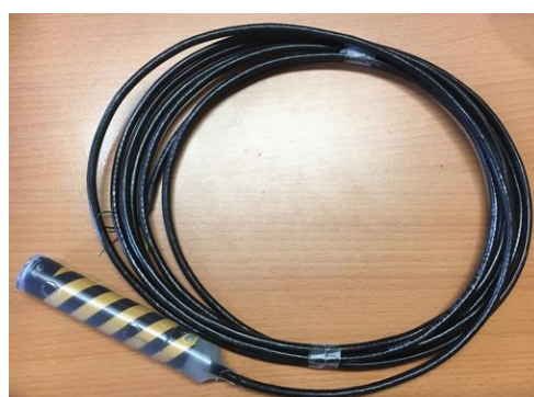
Figure 24. Photo of the industrially moulded sensor
