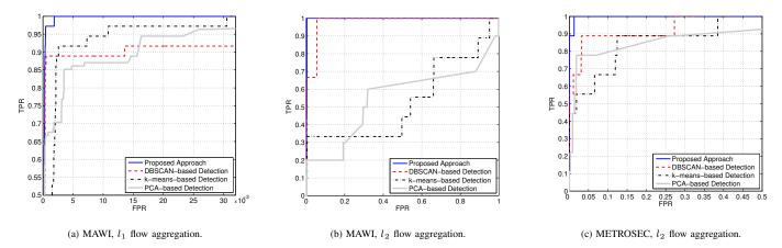
Fig. 6: True positives rate vs false alarms in MAWI and METROSEC. Comparison to state-of-the-art unsupervised approaches for anomaly detection.
