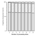
Fig. 9: Proportion of execution time for source aggregated flows clustering (vertical stripes), destination aggregated flows clustering (diagonal stripes) and other processing time (horizontal stripes), according to an increasing number of processing slices.
