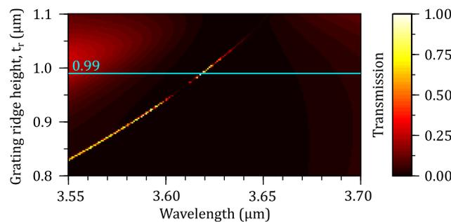
FIG. 3. Transmission spectrum as a function of the grating ridge height  $t_g$ . The light blue line corresponds to the case  $t_r = 0.99 \mu\text{m}$ , taken as reference for the rest of the study. The fixed device parameters are as follows:  $t_s = 0.22 \mu\text{m}$ ,  $\Lambda = 1.255 \mu\text{m}$  and  $f\Lambda = 321.3 \text{ nm}$ .
