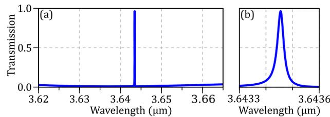
FIG. 5. (a) Transmission spectrum for a particular highly-resonant filter using *Ge* slab and grating above a *ZnS* substrate, with (b) a zoom in the vicinity of the transmission peak. At the resonance wavelength of the transmission peak ( $\lambda = 3.6435 \mu\text{m}$ ):  $n_{Ge} = 4.173$  et  $n_{ZnS} = 2.164$ . The dimensions of the filter are the following ones:  $t_s = 0.198 \mu\text{m}$ ,  $t_r = 1.02 \mu\text{m}$ ,  $\Lambda = 1.255 \mu\text{m}$  and  $f\Lambda = 321.3 \text{ nm}$ .
