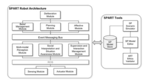
Figure 1. SPART-RA Architecture and SPART Tools.
