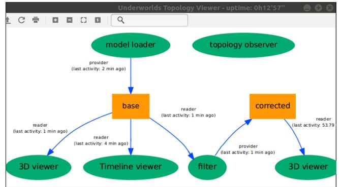
Fig. 4. Screenshot of the network topology introspection tool, with arbitrary examples of worlds (represented as boxes) and clients (ellipses). Clients are connected to the worlds either as *readers* or *providers* of data. UNDERWORLDS introspection features make it possible to also visualise when clients were last active.
