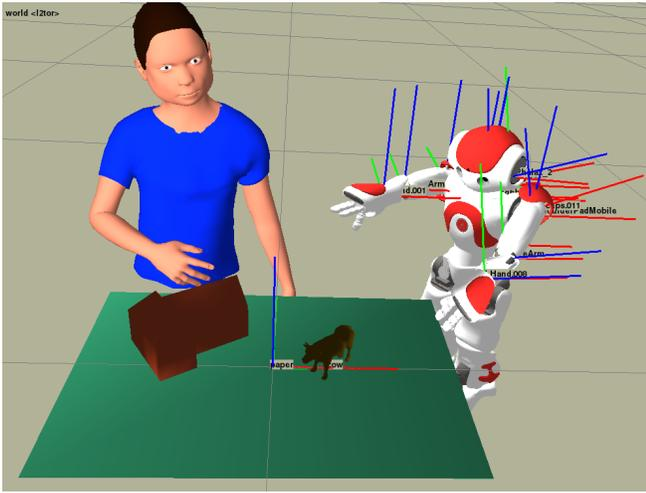
Fig. 3. Screenshot of the `uwds view` 3D visualization and manipulation client. In this particular example, the 3D meshes have been pre-loaded using `uwds load`. Their positions are then updated at run-time using the robot’s sensors and proprioception (joint state).
