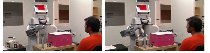
Fig. 4. The same experiment as in fig. 3 described in section V-A was held on the PR2 robot (the robot needs to place the three objects accessible to the human). The environment was set, then a plan (both at symbolic and geometric level) was computed by our algorithm and finally executed (the execution part is not a contribution of this paper).
