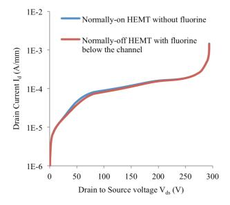
Fig. 8. Simulated  $I_d(V_{ds})$  characteristics in the off-state, showing the off-state current and the breakdown voltage of the normally-on HEMT and the normally-off HEMT with fluorine implantation below the channel.
