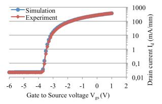
Fig. 2. Comparison of experimental and simulated  $I_d(V_{\rm gs})$  transfer characteristics showing a clear match for the threshold voltage and transconductance.
