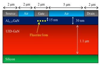
Fig. 4. Schematic cross-section of the simulated HEMT with fluorine implanted in the AlGaN layer.
