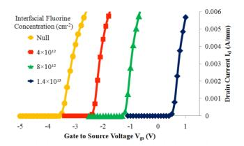
Fig. 3.  $I_d$  (V\_{gs}) transfer characteristics of the conventional normally-on HEMT and HEMTs with fluorine implanted in AGaN at various concentration.
