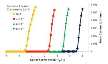
Fig. 5. I<sub>d</sub> (V<sub>gs</sub>) transfer characteristics of the conventional normally-on HEMT and HEMT with fluorine implanted in GaN at various concentration.
