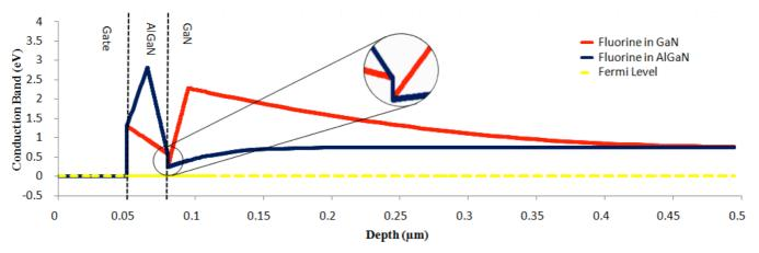
Fig. 7: Band diagrams of HEMT with fluorine implanted in AlGaN at concentration  $1.4 \times 10^{13}$  cm<sup>-2</sup> and HEMT with fluorine in GaN at concentration  $8 \times 10^{12}$  cm<sup>-2</sup>; both HEMTs attain a threshold voltage of 0.5 V.
