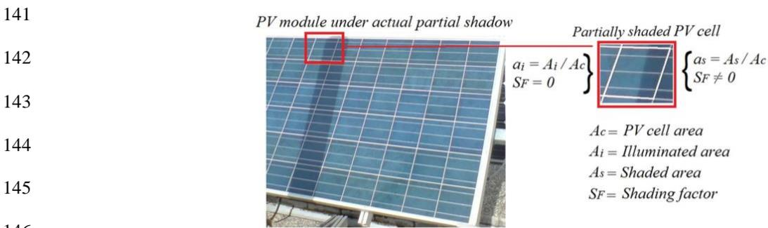
147 **Fig. 1 : Partially shaded PV cell**
