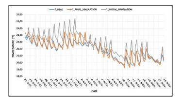
Fig. 4. Example of model calibration for an office during a 1-month period
