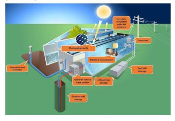
Fig. 2. Energy Systems installed in the ADREAM Building
