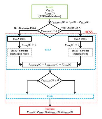
Fig. 2. Flow chart diagram of HESS simulation algorithm in LVDC-MG
