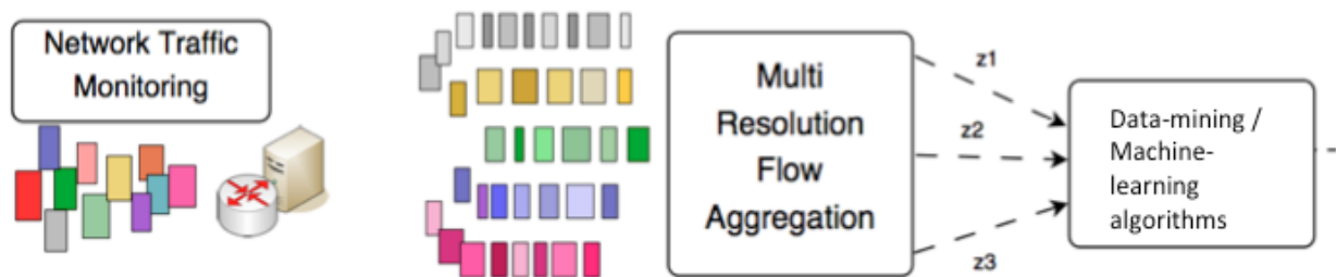
Figure 3: Traffic pre-processing for scalable online characterization
