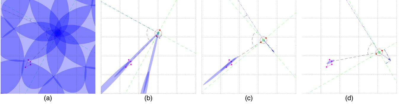
**Fig. 3.** Audio-motor localization of a loudspeaker (top right edge of the pentagon) by a moving spherical binaural head. (a): Self-initialization. (b): Front-back ambiguity when no head motion. (c)-(d): Disambiguation thanks to the head motion.
