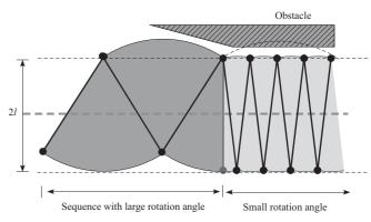
Fig. 9 The swept volume of pivoting. It converges to the swept volume of the supporting edge along the straight line segment by reducing the rotation angles. Therefore, the original collision-free Reeds and Shepp path can be converted into a collision-free pivoting sequence.
