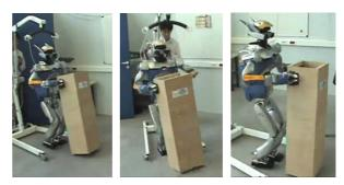
Fig. 2 An experiment of whole-body pivoting manipulation.
