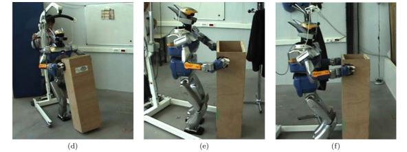
Fig. 14 Experimental results. Starting from the initial position (a) with obstacle at right-hand side, the humanoid robot manipulates the object backwards away from the wall (b). After switching motion direction to forward (c), the robot continues to manipulate the object to the goal position by avoiding the obstacle (d-f).
