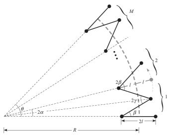
Fig. 8 Transforming an arc of circle path into a pivoting sequence. The regular sequence is composed of symmetric rotations. The center of pivoting line segment arrives at the end point of the arc with the perpendicular orientation.
