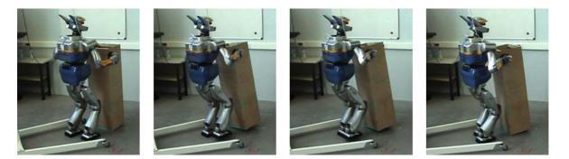
Fig. 15 Detailed whole-body pivoting motion in backward direction. Starting from the initial configuration, the humanoid robot makes coordinated leg and arm motions. The robot rotates the object clockwise by supporting it on the left corner and stepping back with right leg.
