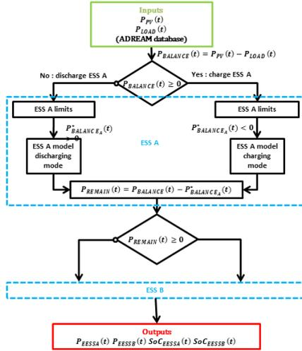
Fig. 2 : Flow chart diagram of HESS
