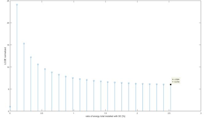
Fig 3: HESS LCOE for different values of SCs
