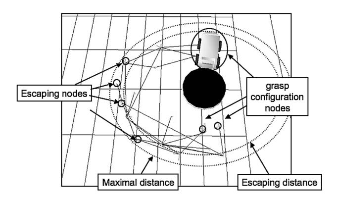
Figure 5: The Relative Roadmap that encodes several approach and contact paths of *forklift* relatively to a cylindrical object.
