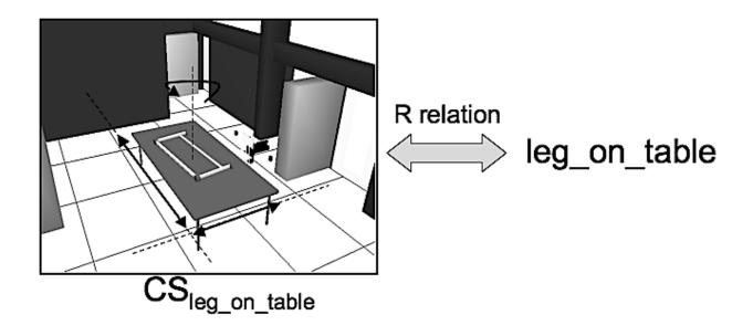
Figure 2: An example of  $\mathcal{R}$  relation. Here  $cs_{leg\_on\_table}$  is a three-dimensional sub-manifold including the configurations (positions and orientations) that correspond to a stable placement of the leg on the table.
