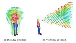
Fig. 2. The costmaps model the distance and visibility constraint by assigning to each point of the cartesian space an HRI cost. The safety cost function is inversely proportional to its distance to the human while the visibility cost function reasons about the field of view modeled by the gaze direction.
