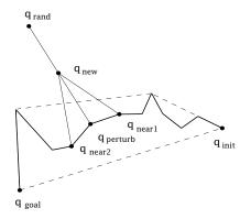
Fig. 5. The random path perturbation does not restrict the new path to be inside the convex hull defined by the path's set of points enabling a more global exploration of the input path neighborhood.
