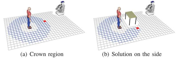
Fig. 5. The estimated handover positions of the robot, feasible (in blue) and closest feasible  $cell_{min}$  (in red) for a given human position according to the reaching capabilities of the human and the robot.
