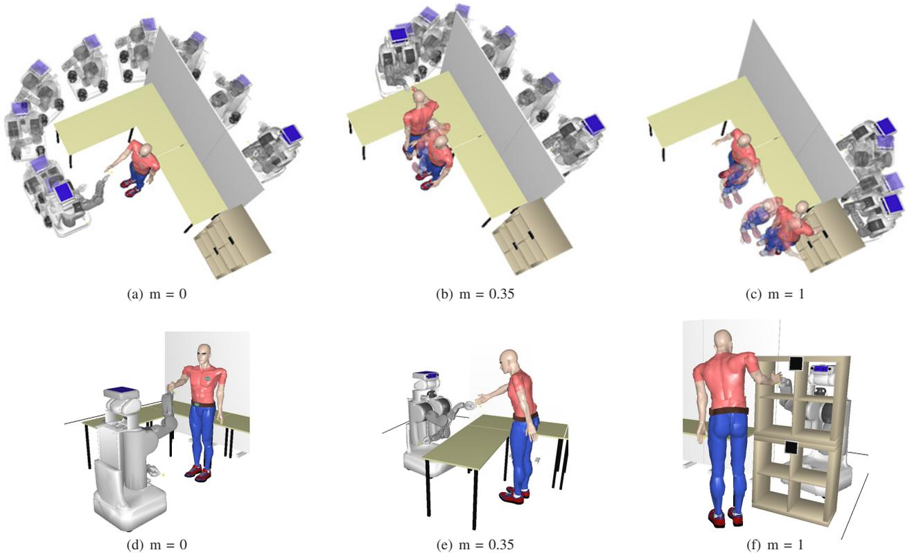
Fig. 6. Three values of the *mobility* parameters are used to generate three handover strategies. The first three pictures depict the resulting trajectories while the three bottom pictures show the final handover configuration that accounts for the 3D obstacles.
