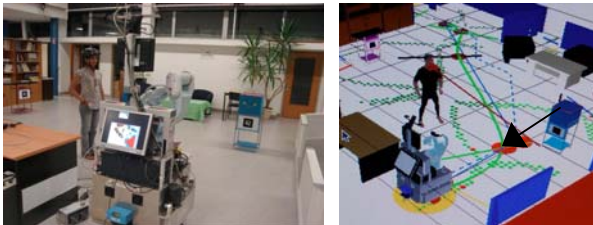
Fig. 8. Crossing a standing person, avoids entering into personal space. the person from her left side. Fig. 6(d) (e) show the current state of the environment which robot is maintaining and the black arrows show the initial and the modified path of the robot after it has predicted that even if there is no direct collision it might enter into personal space of the human. Fig. 7 shows the case where robot has suspended the social convention of passing by, as the clearance was not sufficient on the left side of the person. Instead the robot has modified its path to pass by from the right side of the human for avoiding entering into the personal space. Fig. 8 shows the case when the human is not moving. Robot has planned the path, shown as black arrow, to smoothly cross the person to reach the goal, while maintaining the proximity constraints around the person.
