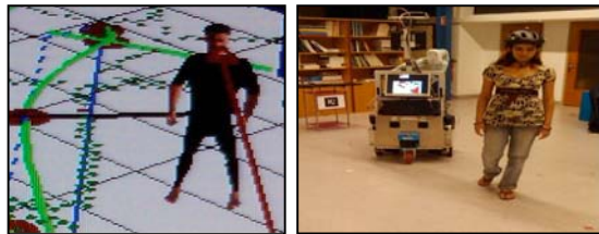
Fig. 7. Suspending the social convention of passing by from left and passing from right side because of insufficient clearance on the left side of human.
