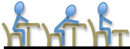
Fig. 3. Human closer to the table (a) could lean less compared to sitting away from the table (b). Table is too low to be reached without leaning (c).
