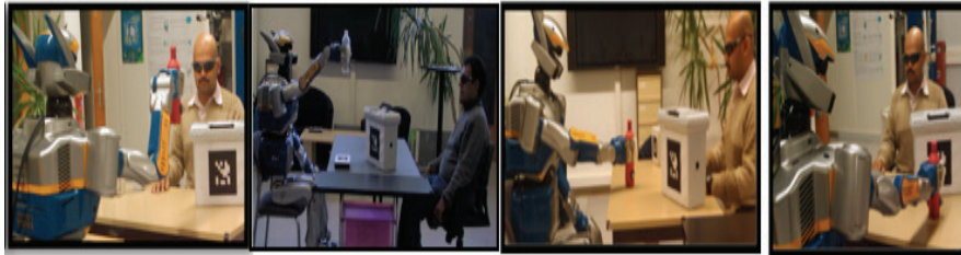
Fig. 11 (a)-(d) (a) and (b) HRP2 showing the bottle to two different humans, (c) reaching and grasping the bottle and (d) hiding it from the human.
