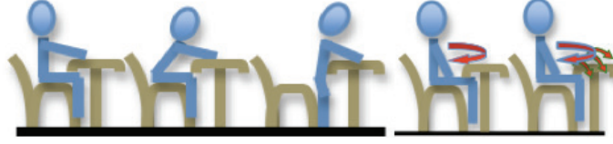
Fig. 2 (a)-(e) Taxonomy of reach actions (a) arm-shoulder reach, (b) arm-torso reach, (c) standing reach. We have augmented the set by (d) turning around reach and (e) turning around and leaning reach.
