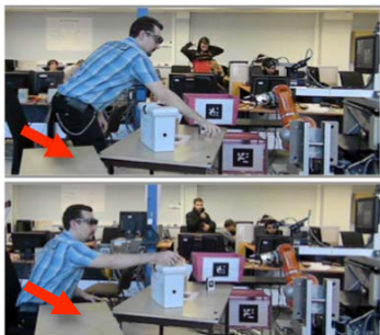
Fig.11: Human makes an object accessible to the robot. (a) In absence of verbal proactive behavior about where to put, human is putting with more effort, Whole_Body_Effort . (b) Human is putting with less effort Arm_Torso_Effort , when robot is proactively saying to put on the box. Red arrows show the initial positions of the object to make accessible.
