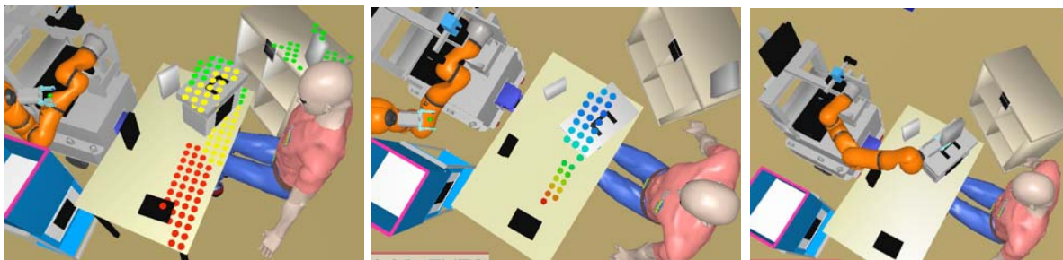
Fig.7: Task of making an object accessible by the human to the robot. (a) Places on the support planes where the human can put the object, by right (green), both (yellow) and left (red) hands. (b) Candidate points where the robot can support human, blue has the highest weight requiring least effort from human. (c) Robot anticipates possible placement of the object on the box, from where it is feasible to take, while ensuring least effort from the human.
