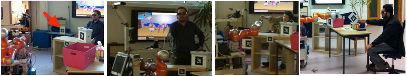
Fig.8: (a) Initial scenario for giving the object marked by red arrow. (b) The human is trying to give it to the robot by standing, Whole Body Effort , in the absence of proactive reach by the robot. In presence of proactive reach by robot’s arm (c) the human is giving it just by leaning forward, Arm_Torso_Effort and (d) giving it by stretching out his arm only, Arm_Effort in a different scenario, where the robot was able to support the Arm_Effort of the human.
