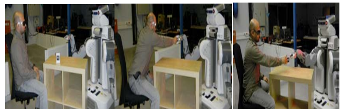
Fig.10: (a) Initial scenario for giving an object by the human to the PR2 robot. (b) The human is putting more effort in the absence of any proactive reach towards object behavior by robot. (c) The human is giving with less effort when robot is reaching out the object proactively.
