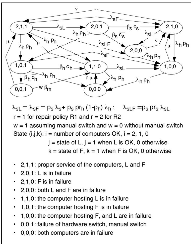
**Figure 9:** Reduced Markov chain of the duplex system
