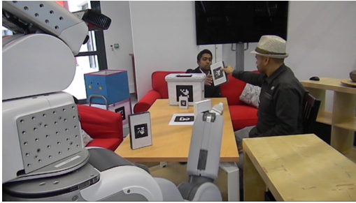
Fig. 9: Execution of Taskability Graph based generated shared plan to give an object to human 1 of fig. 4 by planned help from human 2 , sitting in the middle.
