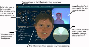
Fig. 5. A view of the interface of the touch-screen.
