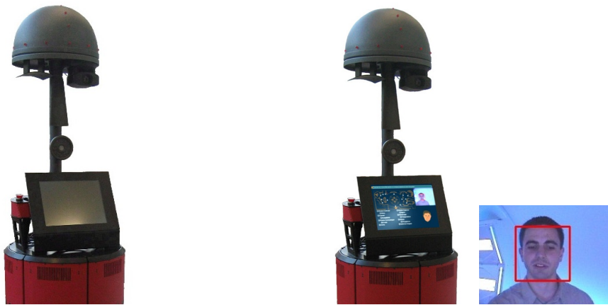
Fig. 3. Rackham sending (or not) feedback to the people via the use of an external representation
