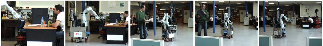
The bottle is not placed in the gripper, simulating a pick-up error.
