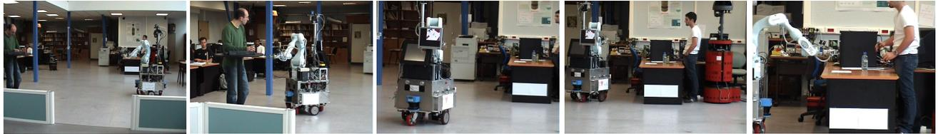
Jido detects a human in its vicinity. A *Bring Object* task is inserted in the plan. Jido starts moving to the human thanks to the MHP motion planner.
