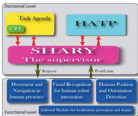
**Figure 1.** Architecture for proactive robots companions: The decisional layer consists of four components. SHARY, which is in charge of task supervision and execution. HATP the planner which provides other decisional abilities, and Task Agenda which manages high-level robot goals in a human and CRS is in charge of the interpretation activity of the persons in the robot vicinity.
