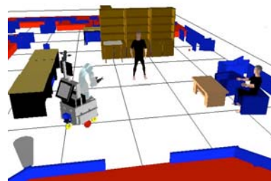
(b) 3D model used by the navigation and manipulation planners
