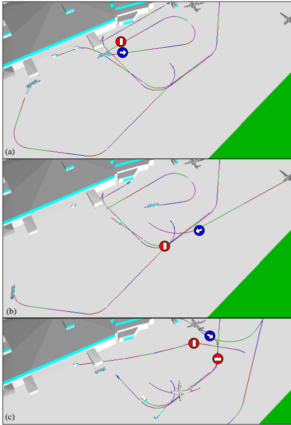
Figure 6: Coordination of two planes, two buses, two trucks and one car in an airport environment. Both planes have the highest priority. Curves on the ground represent the merged plans.
