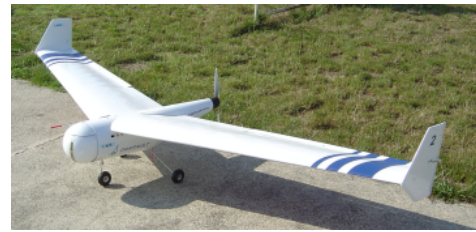
Fig. 8. The UAV Lhasa (3.0 m wingspan, 6.0 kg total)
