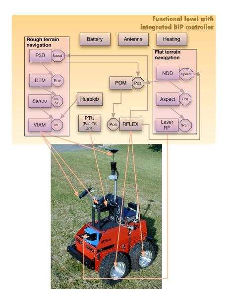
Figure 2: The functional modules of the Dala rover.
