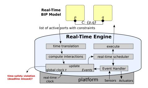
Figure 6: The real-time BIP engine.
