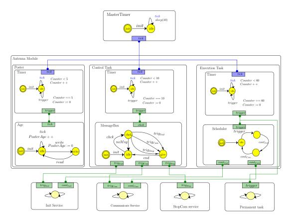
Figure 4: Antenna module implementing timing constraints using ticks.
