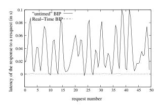
Figure 16: Comparison between real-time BIP and untimed (standard) BIP.
