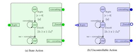
Figure 11: Modelling the robot basic actions using BIP.
