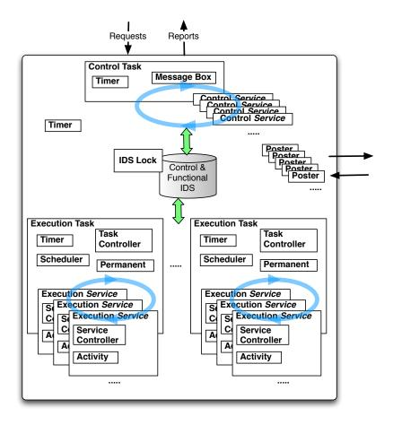
Figure 1: A G<sup>en</sup><sub>o</sub>M module functional organization and its componentization prior to BIP modeling.
