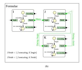
Figure 9: Example of translation: formulae "I meets J and K during J" (a) into a BIP compound component (b).
